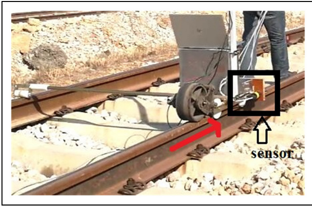
Figure 6. Magnetic sensor signal acquisition.
